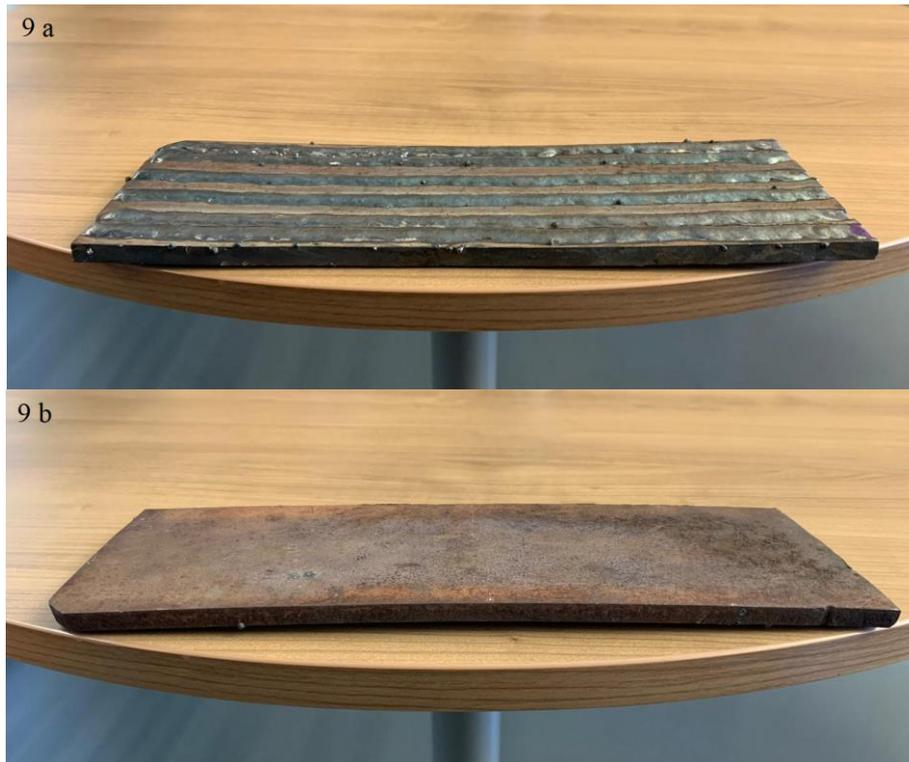
**Figure 9.** a. Hard-faced plate (SIM1) a. upper surface b. bottom surface
