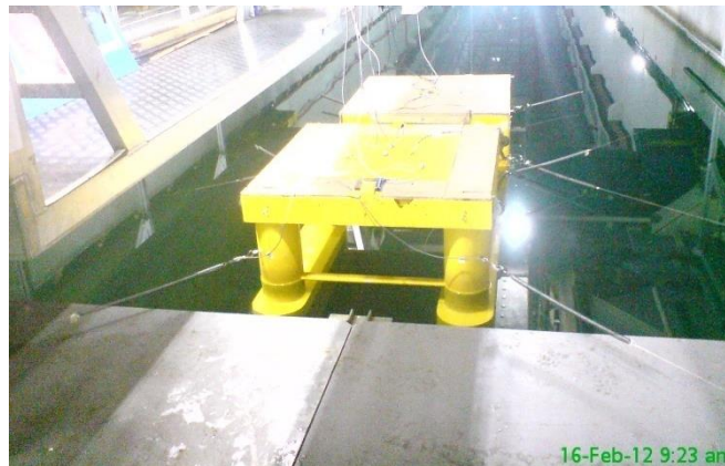
Fig.6 TLP and semi-submersible set up into towing tank.
