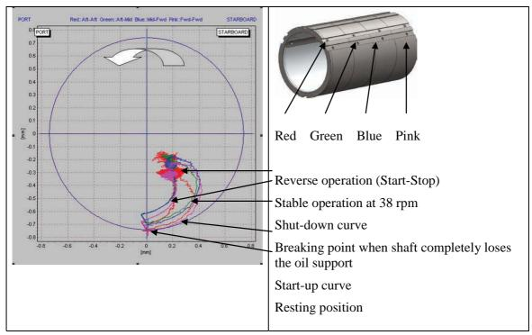
Figure 16 Manoeuvring (astern: start-stop-start- stop)
