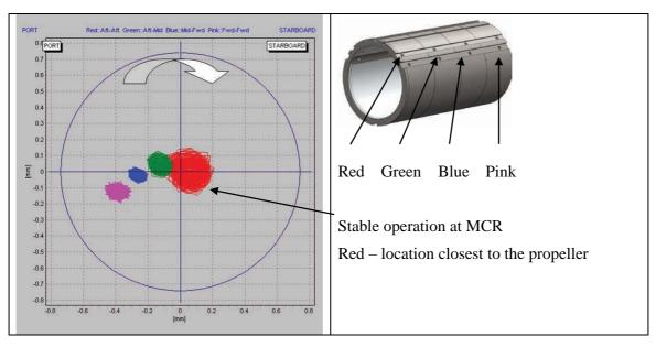
Figure 18 Steady running ahead at rated speed – 112 min<sup>-1</sup>
