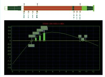
Figure 8 Analytical investigation of the shaft/bearing interaction - propeller shaft with propeller attached
