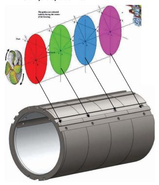
interest is to find the shaft's position relative to the centre of the bearing. The proximity probe measures the distance from the tip of the probe to the closest distance on the shaft. Knowing the bearing/shaft clearance, we can define the shaft position relative to the bearing and observe the interaction between the shaft and the bearing at a particular plane (as in Figure 5).
