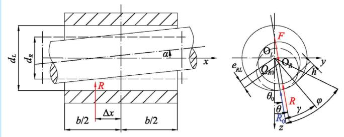
Figure 1 Schematic view of the model of nonlinear radial journal bearing
