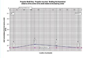
The forward stern tube bearing was not considered in the measurement; however, it is included in the analytical evaluation. In this case, the point contact is obtained on the aft stern tube bearing: two points (forward and aft edge of the bearing), and on the forward stern tube bearing: aft edges of the bush. Distances between the shaft and the bearing are compliant with the analytically predicted position of the shaft.
