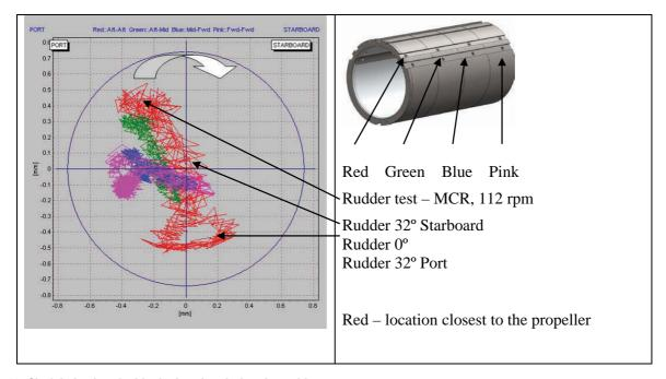
Figure 19 Shaft behaviour inside the bearing during the rudder test
