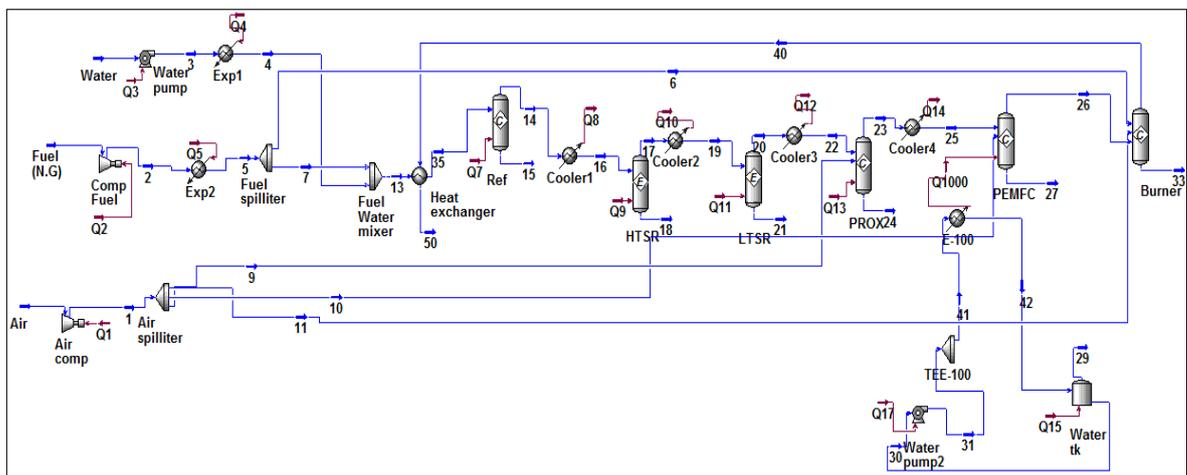
**Fig. 3** Actual steam reforming based PEM fuel cell system flow diagram simulated by Aspen HYSYS 3.2.
