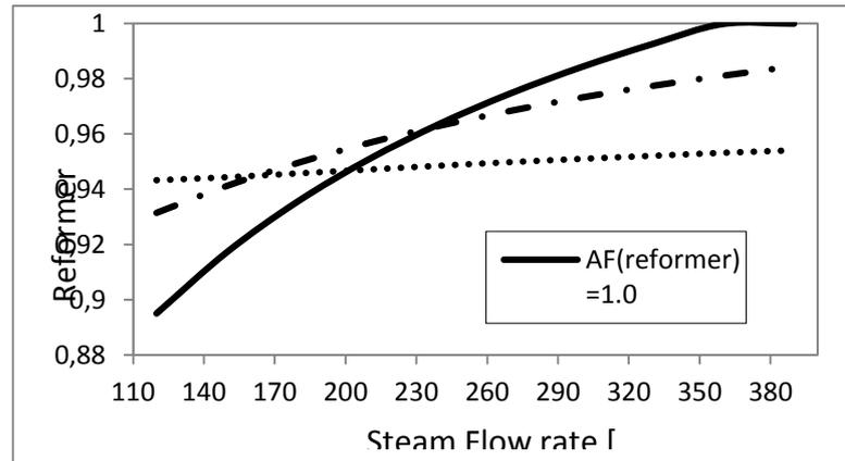
**Fig. 10** Reformer efficiency as a function of steam flow rate and reformer AF ratio (SOFC-PEM)
