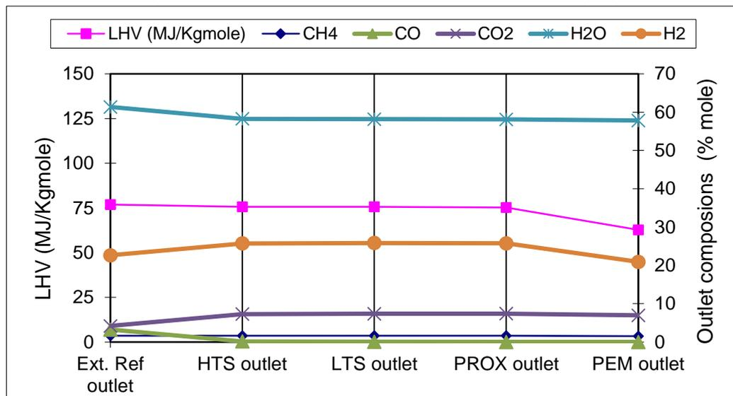
Fig. 7 Product compositions and LHV values of SOFC based fuel preparation reactors.
