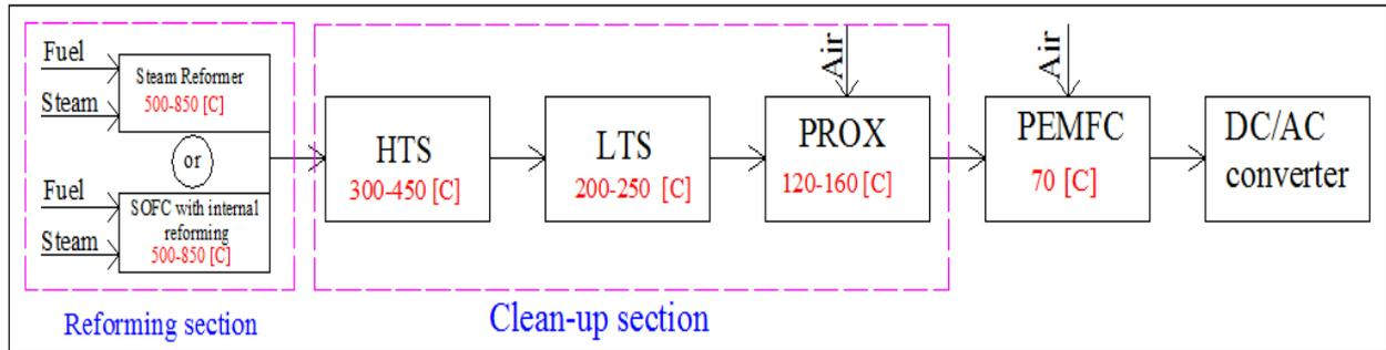
Fig. 1 Typical inlet and outlet steam temperature ranges for PEMFC reactors
