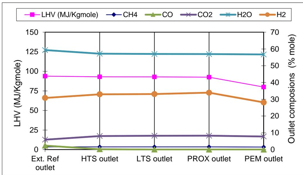
Fig. 6 Product compositions and LHV values of steam reforming based fuel preparation reactors.
