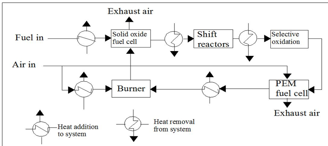
Fig. 2 Reforming option based on solid oxide fuel cell used for PEM fuel cell
