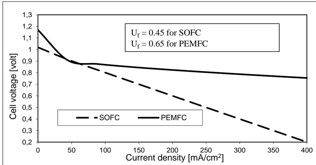
Fig. 5 SOFC and PEMFC polarization curves
