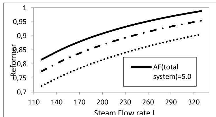
Fig. 9 Reformer efficiency as a function of steam flow rate and total system AF ratio (SREF-PEM)
