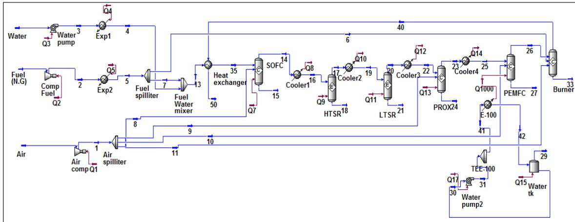
**Fig. 4** Actual SOFC based reforming PEM fuel cell system flow diagram simulated by Aspen HYSYS 3.2.
