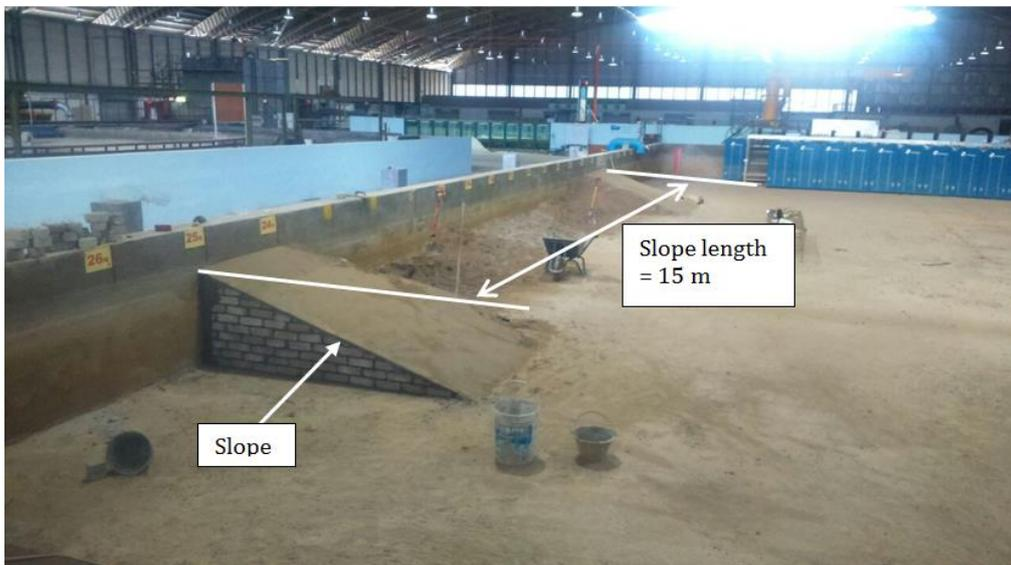
**Fig. 10** Slope setup under preparation at NAHRIM facility for model testing
