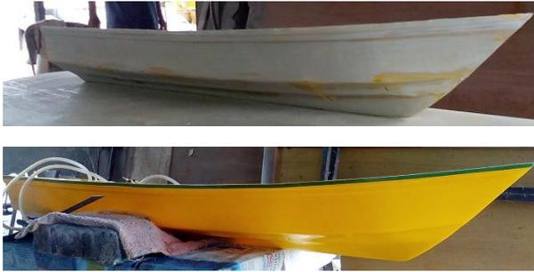
**Fig. 8** Construction of the model hull form
