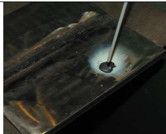
**Fig. 5b** Damage repair by welding
