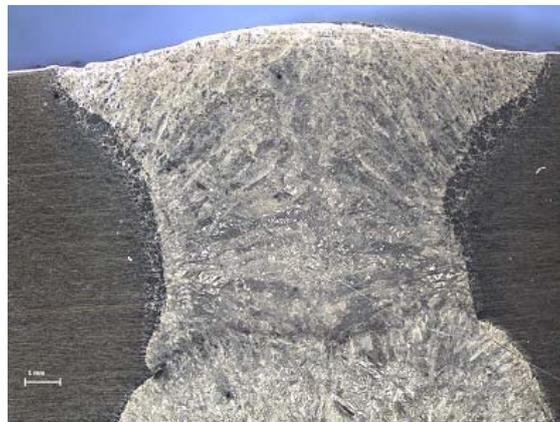
**Fig. 7** Macrostructure of the welded joint
