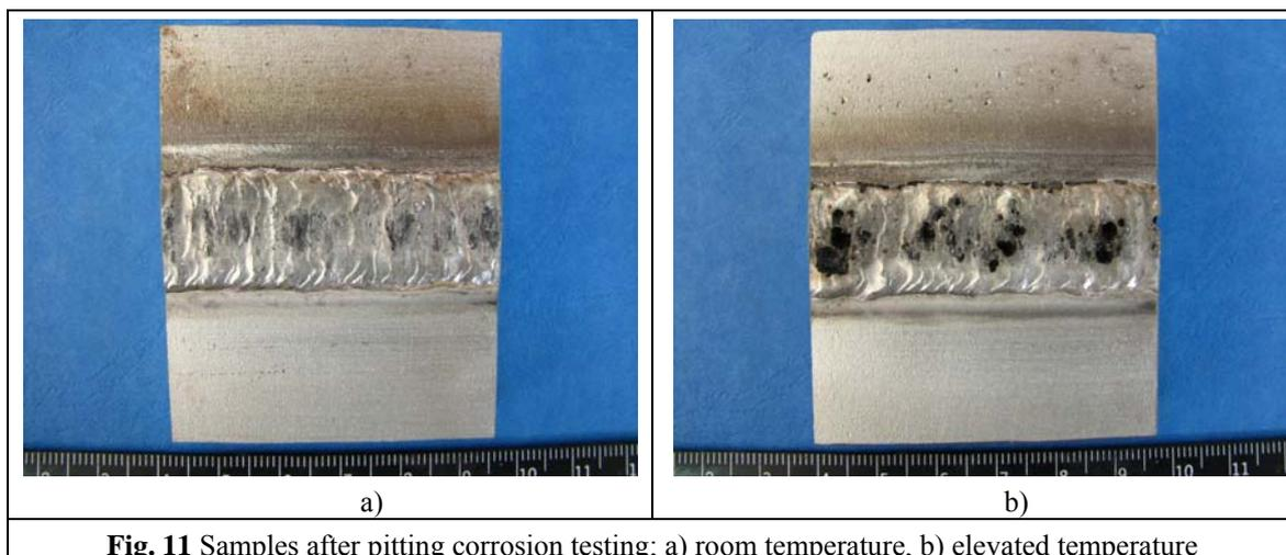
**Fig. 11** Samples after pitting corrosion testing; a) room temperature, b) elevated temperature
