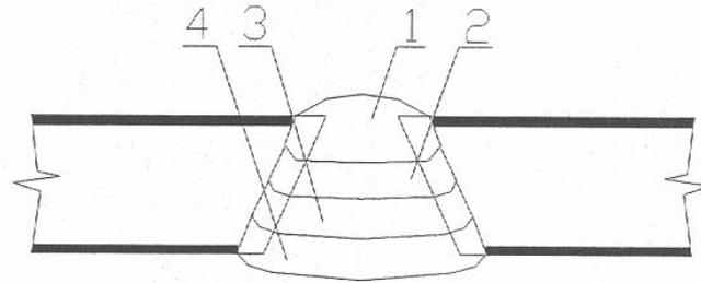
**Fig. 4** Four passes butt welded joint
