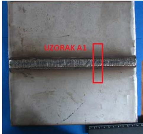
**Fig. 6** Testing strips cutting scheme
