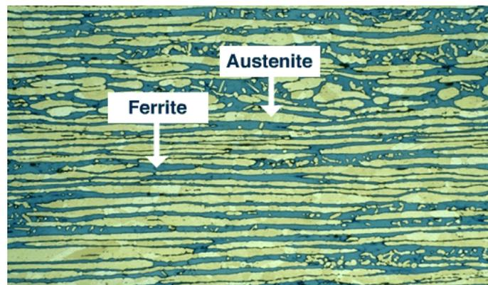
**Fig. 3** The microstructure of duplex stainless steel [7]
