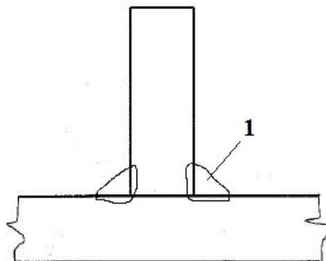
**Fig. 13** Fillet joint scheme
