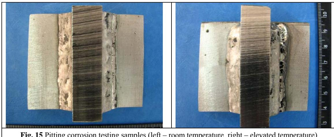
**Fig. 15** Pitting corrosion testing samples (left – room temperature, right – elevated temperature)
