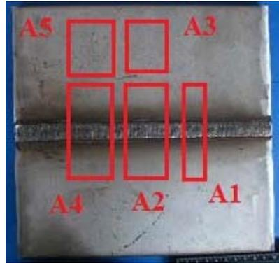
**Fig. 10** Cut samples locations for pitting corrosion resistance testing
