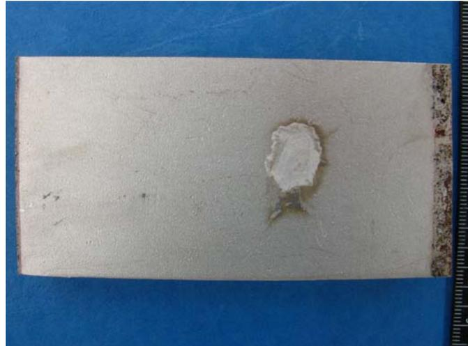
**Fig. 12** Pitting corrosion on repaired part of the material – elevated temperature
