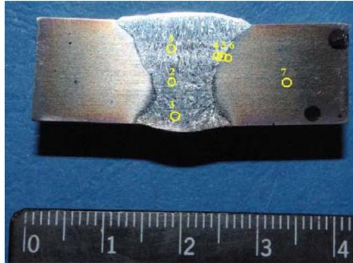
**Fig. 8** Butt weld joint microstructural locations testing
