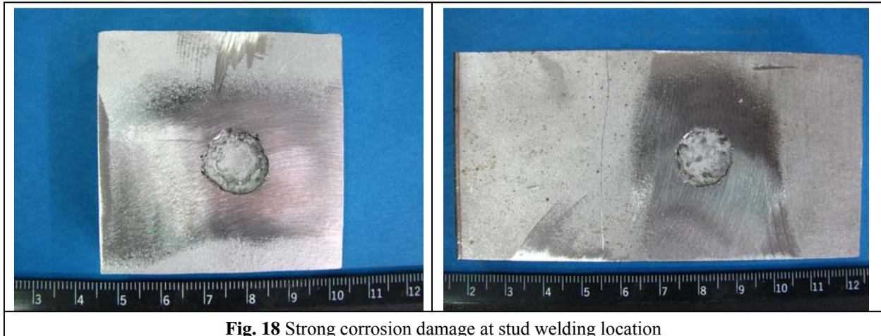
**Fig. 18** Strong corrosion damage at stud welding location
