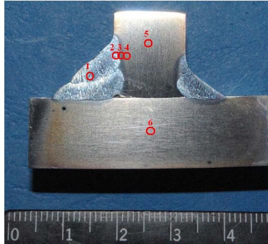
**Fig. 14** Locations (1-6) for fillet joint microstructure testing
