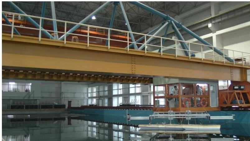
Fig. 12 Process of trimaran model test
