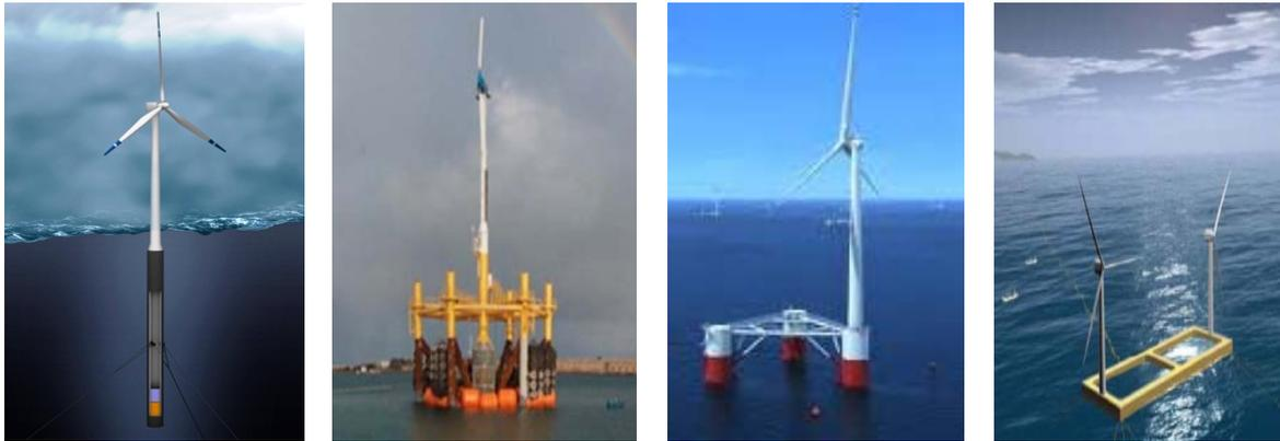
**Fig. 10** Prototype (a) spar-type wind turbine and (b) TLP type wind turbine (c) semi-submersible type wind turbine and (d) pontoon type wind turbine (Wang et al. (2010)).
