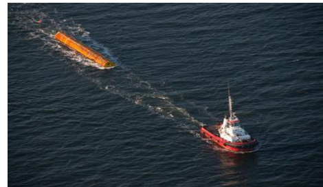
Fig. 11 Transporting offshore wind foundation to site
