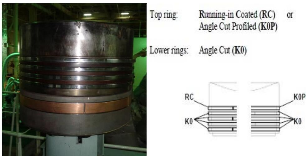
**Figure 1.** Design and configuration of the piston rings
