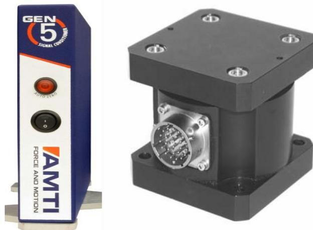
Fig. 6 AMTI load cell and amplifier.
