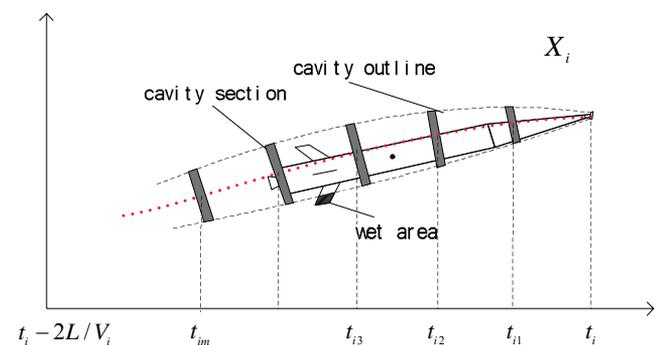
At each discretized node, estimating time intervals  $\{[t_i - 2L/V_i, t_i]\}$ ,  $i = 0, 1, \dots, N$  with certain number of sampling points  $m$  is established. Based on the cavitator track, motion states at each  $t_{ij}$  ( $j = 1, 2, \dots, m$ ) are interpolated to calculate the real time cavity sections which define the accurate cavity shape and the wet condition of the vehicle (see Figure 5).
