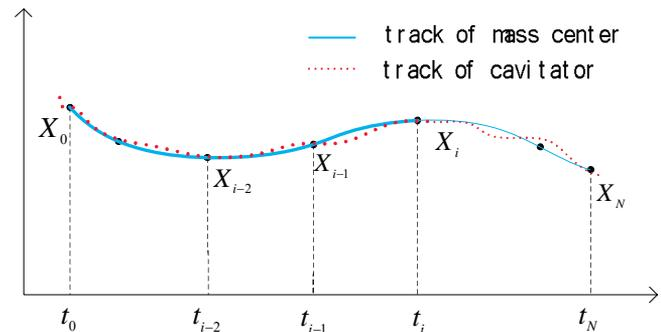
Figure 4 Tracks presentation of vehicle mass centre and cavitator
