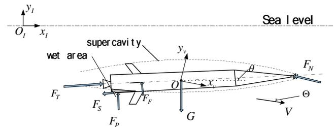
Figure 2 Forces acting on supercavitating vehicle
