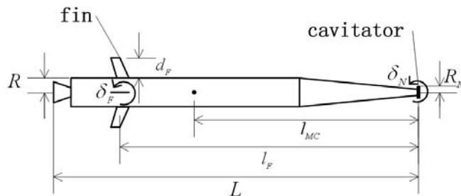
Figure 1 Configuration of supercavitating vehicle
