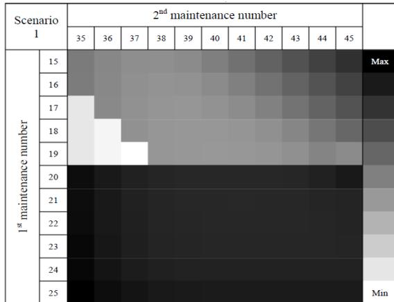
**Fig. 10** Heat map of FOC over time for hull cleaning (scenario 1)
