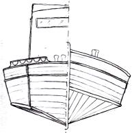
Figure 7 The combined (mixed) building method
