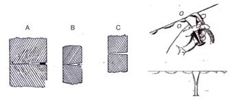
Figure 19 Caulking of boat side shell plating (A- correct joining; B and C incorrect joining)
