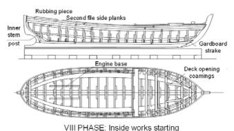
Figure 17 **The eighth construction phase**Slika 17 **Osma faza gradnja**
