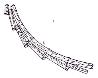
Figure 2 The overlapping planks method (Clinker-method)
