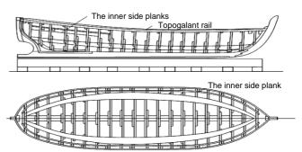
VI PHASE: The gardboard - strakes and inner side planks positioning
