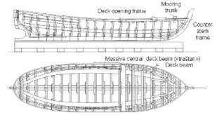
VII PHASE: The deck beams, inner stern frame and deck opening positioning
