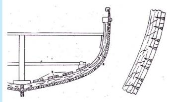
Figure 1 The touching planks method (Carvel-method)
