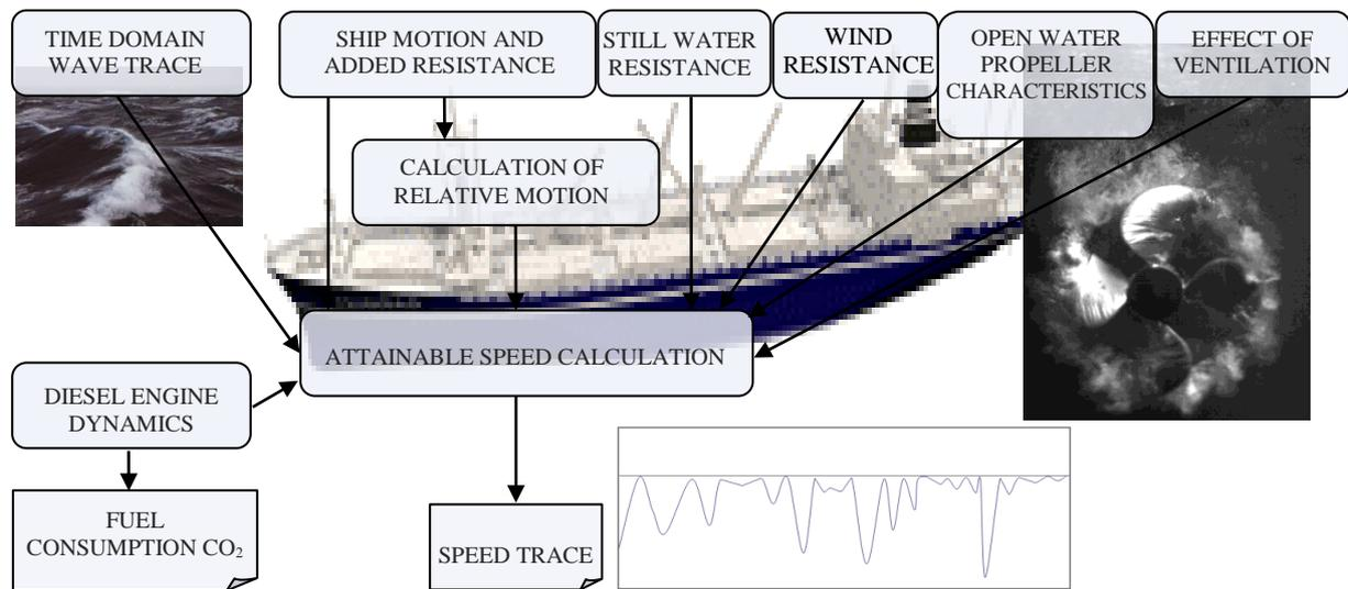
Figure 1. Scheme of the computations of ship speed in a given sea state
