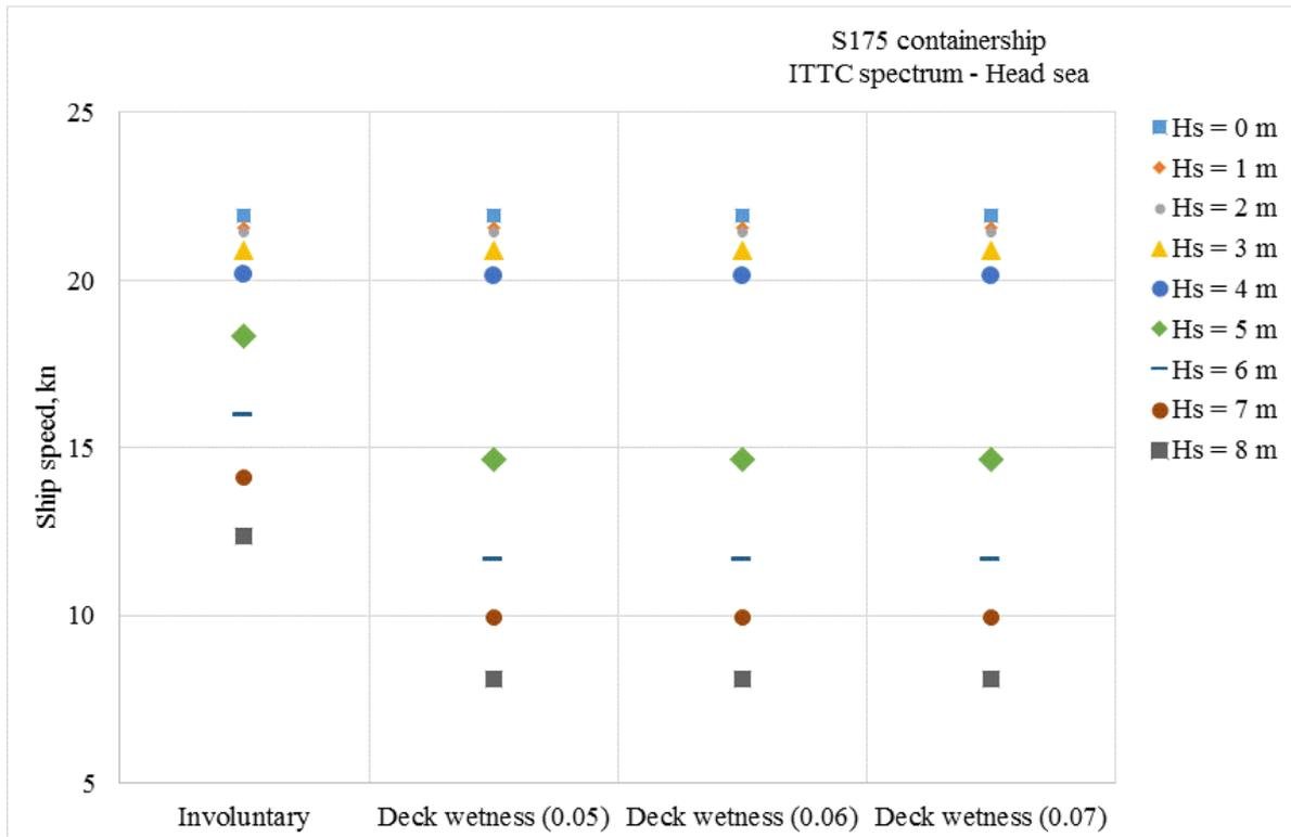
Figure 7. The effect of deck wetness limiting value on attainable ship speed (head sea)
