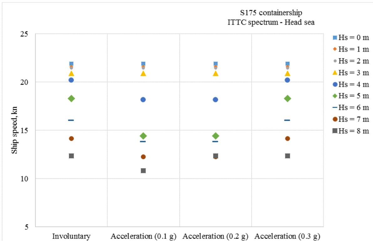
Figure 8. The effect of acceleration limiting value on attainable ship speed (head sea)
