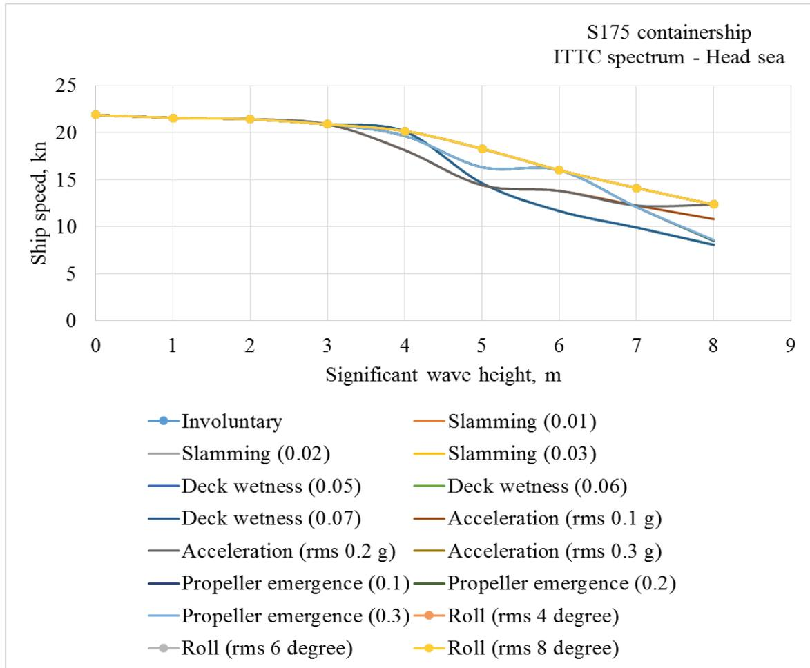
Figure 5. Ship speed loss for head sea
