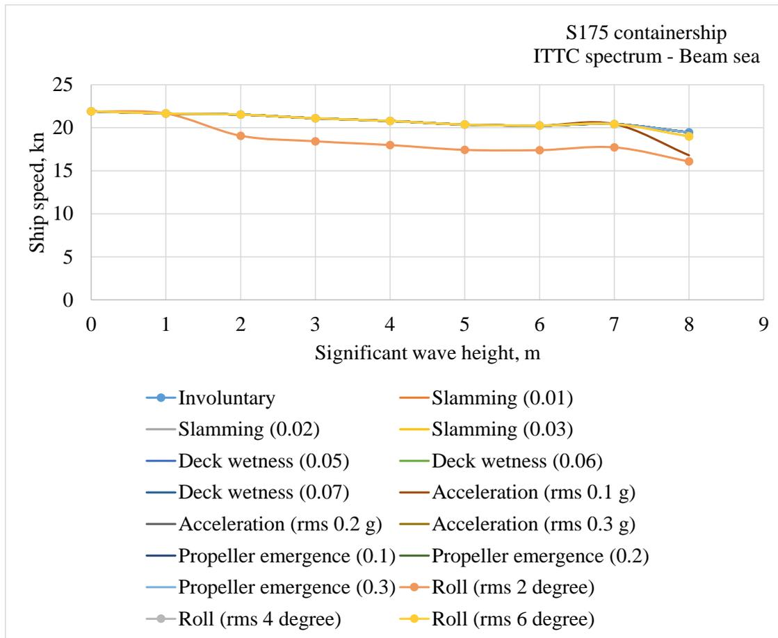
Figure 17. Ship speed loss for beam sea
