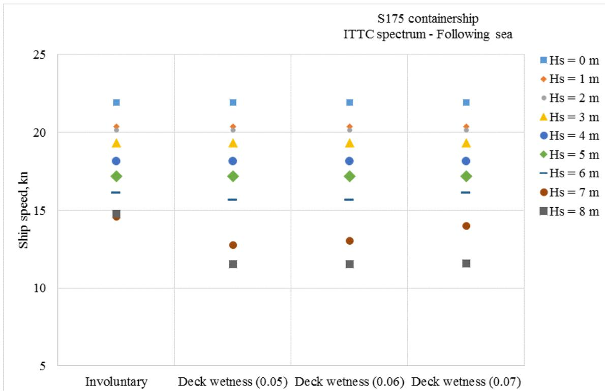
Figure 13. The effect of deck wetness limiting value on attainable ship speed (following sea)
