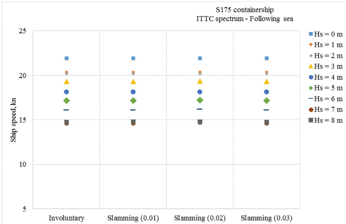
Figure 12. The effect of slamming limiting value on attainable ship speed (following sea)
