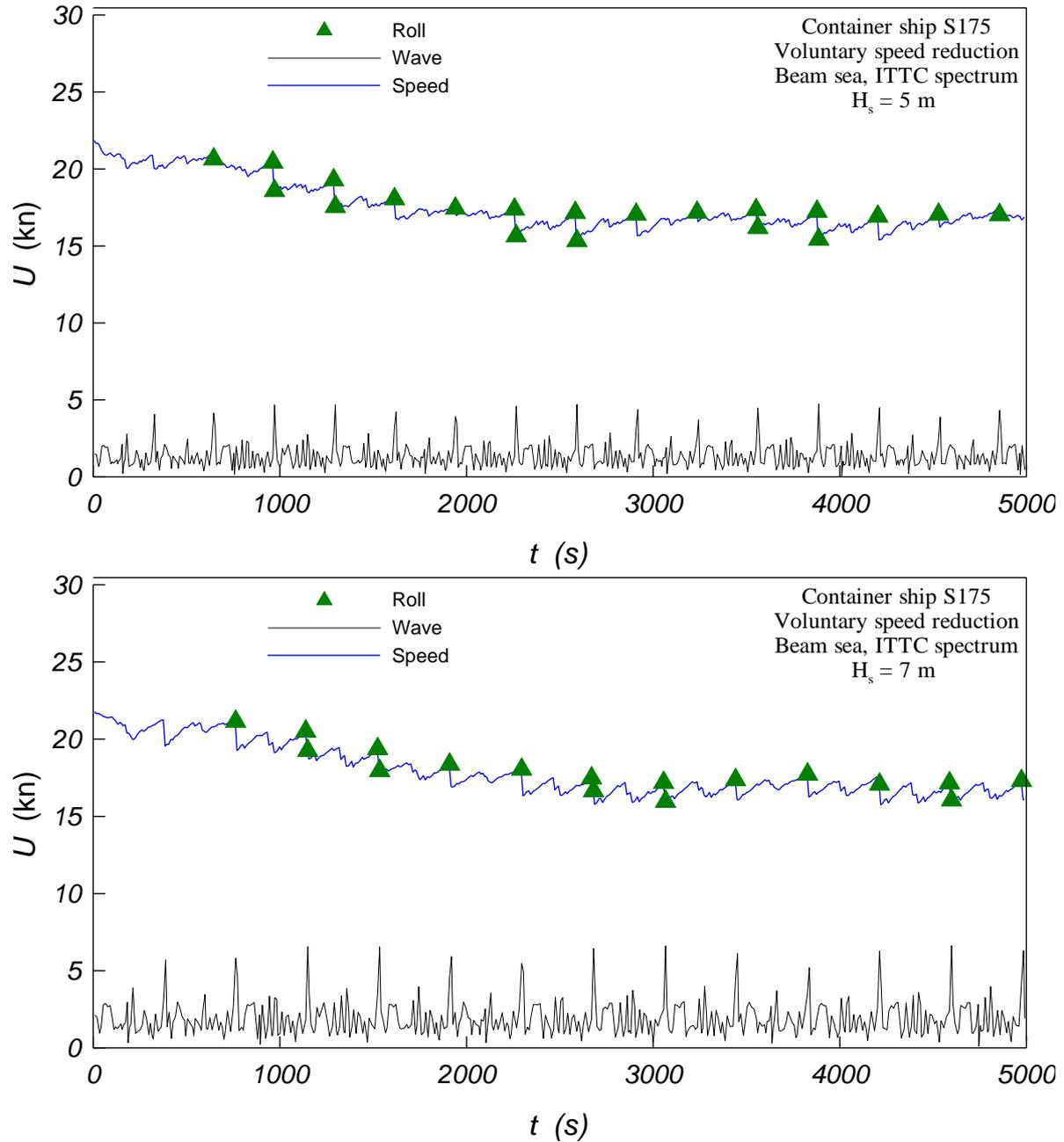
Figure 4. Time trace of ship speed in beam sea
