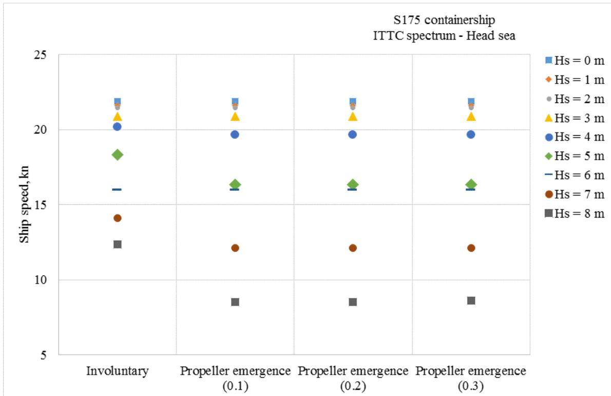
Figure 9. The effect of propeller emergence limiting value on attainable ship speed (head sea)
