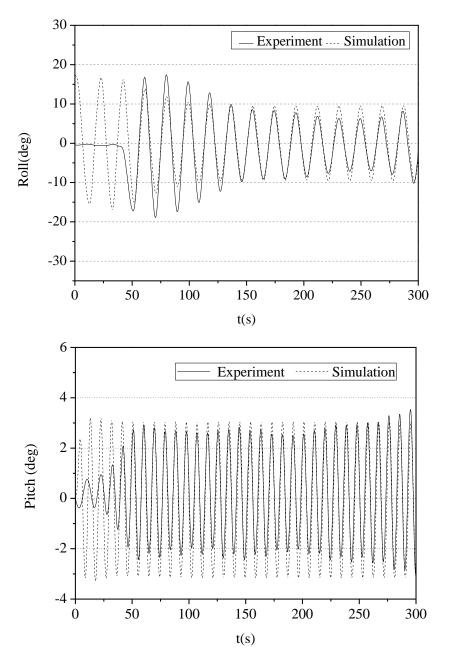
Fig.11 Comparison of time history between experimental measurements and numerical simulations, Fn=0.15,  $H_w$ =7.86m
