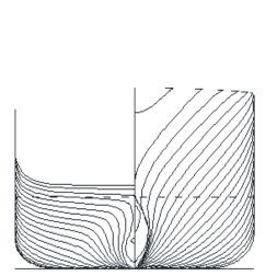
Fig. 3 Lines plan for the C11 containership
