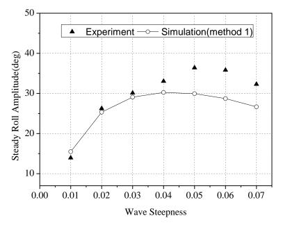
Fig.14 Illustration of the nonlinear stiffness/hardening effect for the C11 Containership in head waves, Fn=0.05
