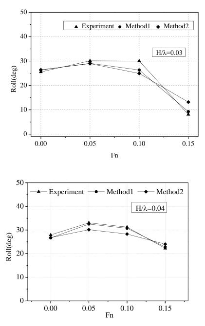
**Fig.13** Comparison of steady roll amplitudes between experimental measurements and numerical simulations using different roll damping prediction methods for the incident wave steepness H/ $\lambda$ =0.03,0.04.
