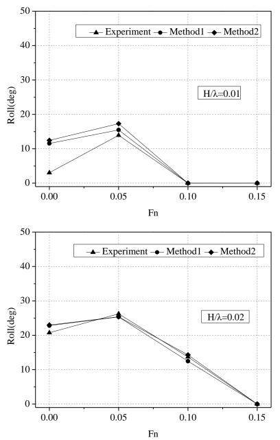
Fig. 12 Comparison of steady roll amplitudes between experimental measurements and numerical simulations using different roll damping prediction methods for the incident wave steepness H/  $\lambda$  =0.01, 0.02.
