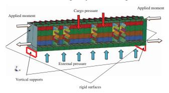
Figure 16 A 3D FE model of the chemical tanker Slika 16 3D MKE model tankera za kemikalije
