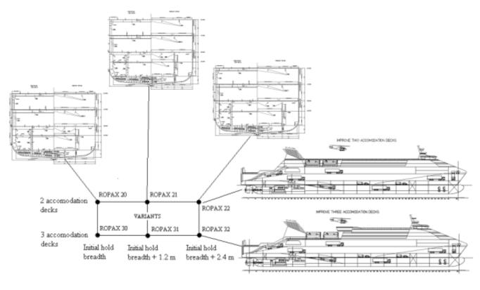
FEM models, see [21], in the generation of design alternatives on the Pareto frontier. In Ro-Pax case, they were further validated using the *IMPROVE* developed adequacy and quality measures (fatigue, robustness, LCC and production cost).
