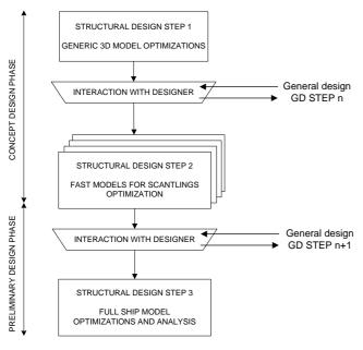
Figure 10 Overall design procedures Slika 10 Projektni postupak
