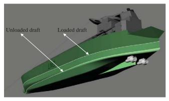
Figure 6 New concept of a 'two-draft' ship, using minimal or no ballast in the unloaded condition
