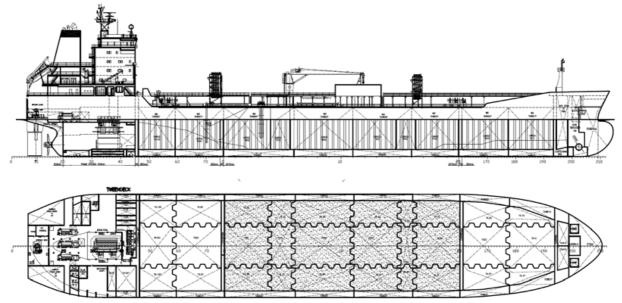
Figure 13 A 40 000 DWT chemical tanker designed by SSN Slika 13 40 000 DWT tanker za kemikalije - projekt SSN
