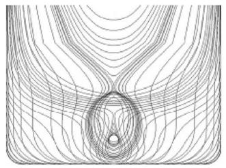
Figure 14 Body plan of the chemical tanker Slika 14 Nacrt rebara tankera za kemikalije
