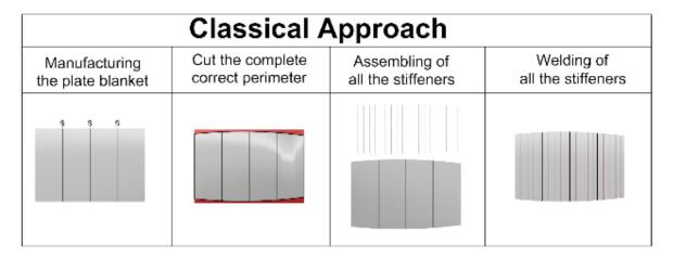
Figure 3 Panel assembly line classical approach sequence
