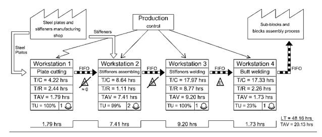
Figure 13 First sequence modification value stream map
