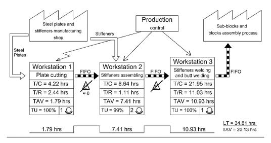
Figure 15 2<sup>nd</sup> sequence modification value stream map
