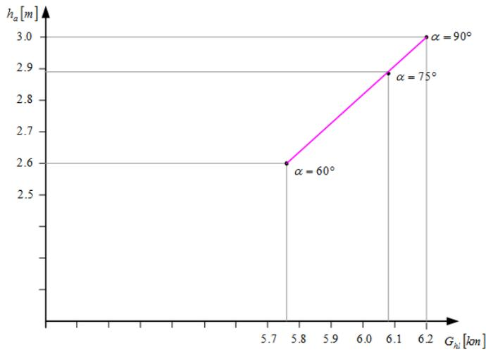
$G_{hl}$  – horizon along the curvature arc;  $h_a$  – height of aerial;  $\alpha$  – angle of rolling
