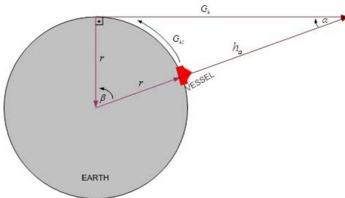
Figure 1 Geometric horizon ( $G_h$ )
