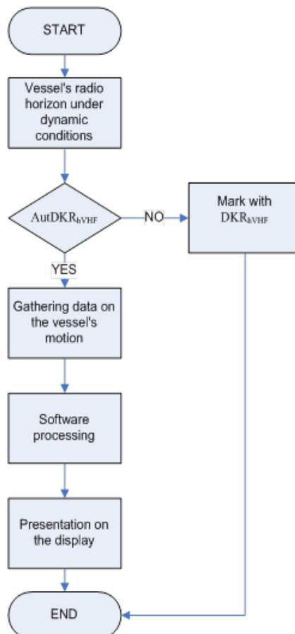
Figure 5 **Algorithm for operation of the automated system ( $AutDKR_{hVHF}$ )**
