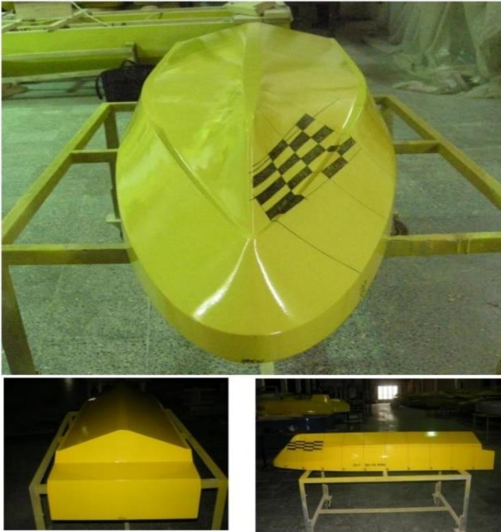
**Fig. 4** The wooden hull model.
