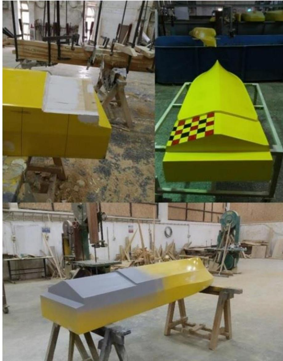
**Fig. 9** Model hull step creation work [32]
