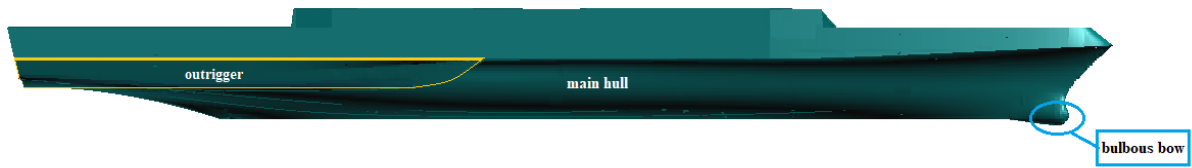
Fig.4 Three-dimensional design of trimaran
