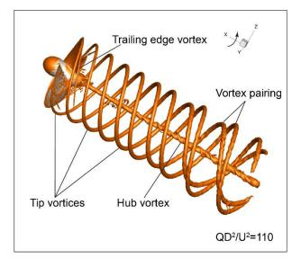
Fig. 6. The instantaneous three-dimensional vortex system behind the propeller represented by the iso-surface of Q=110.
