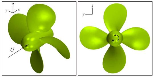
Fig. 1. E779A propeller and reference system.
