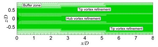
Fig. 3. Mesh distribution with wake refinements including tip vortex refinement and hub vortex refinement.
