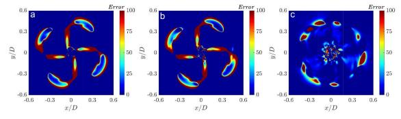
Fig. 20. The contours for (a) reconstruction error of SPDMD, (b) reconstruction error of pi-SPDMD and (c) relative reconstruction error between SPDMD and pi-SPDMD.
