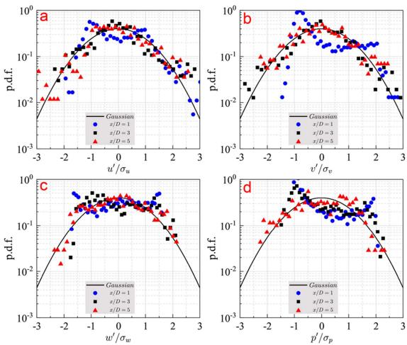
Fig. 11. PDFs of the fluctuations in (a) streamwise, (b) horizontal, (c) vertical velocities, and (d) pressure at downstream probes.  $\sigma$  signifies the standard deviation of the respective flow metric.
