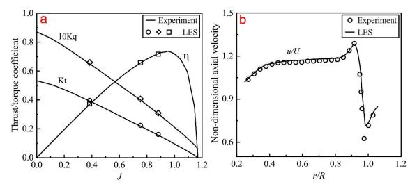
Fig. 5. Comparative analysis of LES and experimental outcomes: (a) open-water attributes and (b) phase-averaged axial velocity at J = 0.88.
