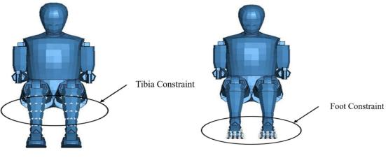
Fig. 7 Dummy tibia constraint
