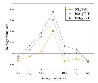
Fig. 23 Corresponding damage ratios for different explosive equivalents
