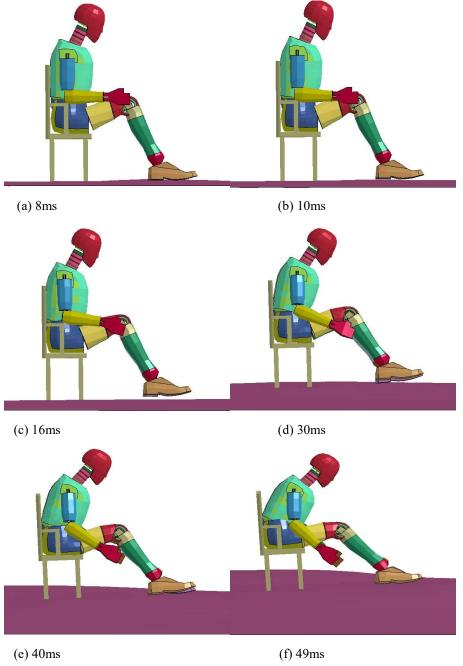
Fig. 13 Posture changes of the dummy at different moments
