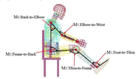
Fig. 6 The Dummy Changes the Joint Posture
