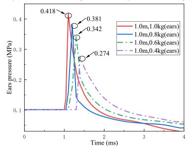
(b) Pressure time course curve at the position corresponding to different explosive equivalents
