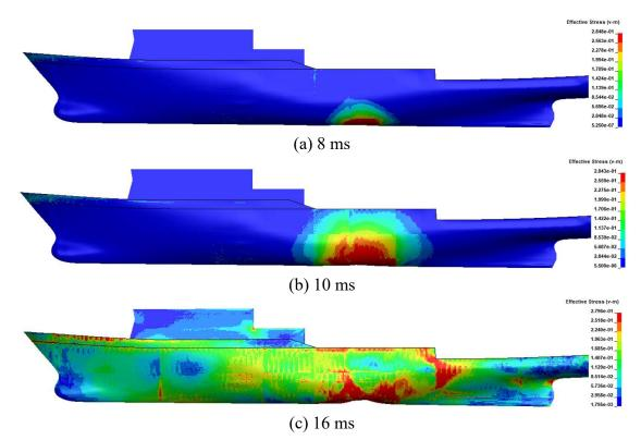
Fig. 11 Response of ship structure under near-field underwater explosion
