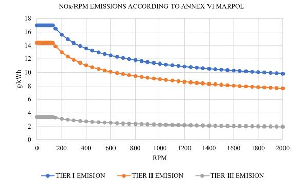
Fig. 10 NO<sub>x</sub> emission curves as a function of RPM according to Regulation 13 of MARPOL Annex VI
