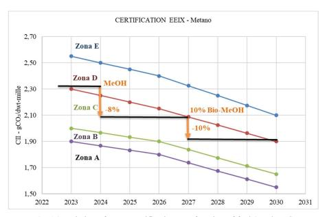
Fig. 16 Variation of EEIX certification as a function of fuel (Methanol)
