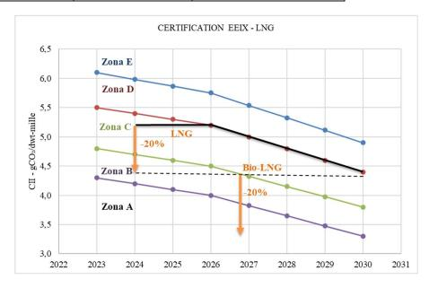
Fig. 15 Variation of EEIX certification as a function of fuel (LNG)
