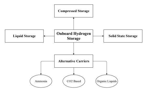
Fig. 3 Onboard hydrogen storage techniques
