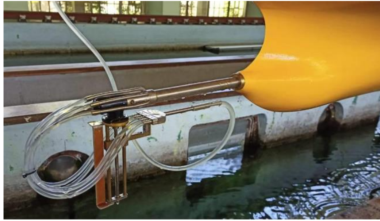
Fig. 2 Five-hole Prandtl Pitot tube mounted behind the stern of the containership model
