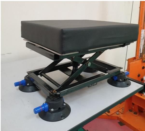
Fig. 4 Retrofittable lightweight prototype suspension seat
