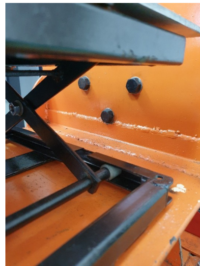
Fig. 5 Replaceable Teflon inside a guide rail of the designed suspension seat
