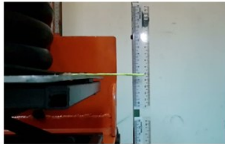
1 st touchdown: point 1 Absolute time: 273.4ms Reading on ruler: 0.046 m Distance travelled: 0.089 – 0.046 = 0.043 m
