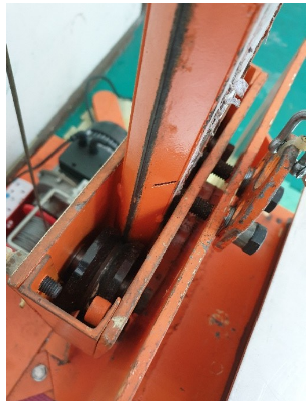
Fig. 3 Roller bearing (2 units) attached to the angle bar (25 mm x 25 mm x 2 units)
