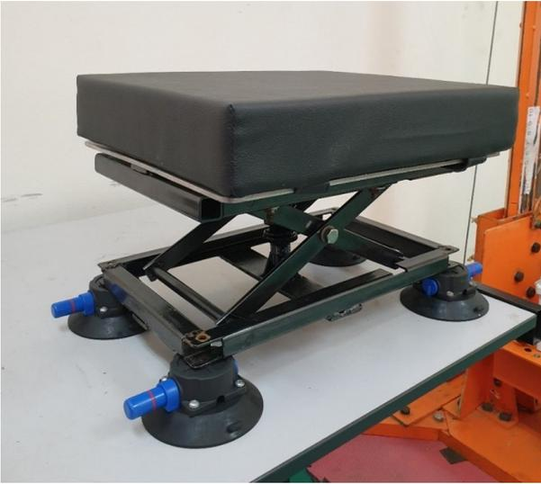
**Fig. 4** Retrofittable lightweight prototype suspension seat
