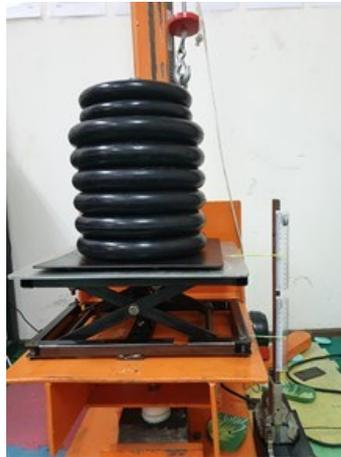
**Fig. 12** Spring stiffness test
