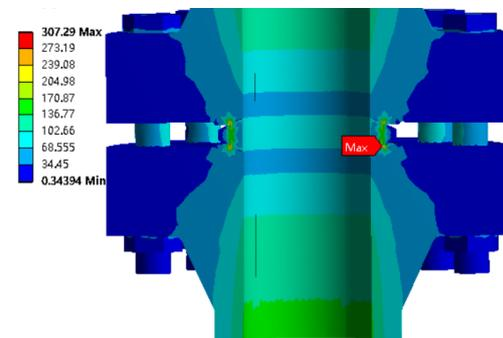
(b) Equivalent stress cloud diagram of the optimized sealing structure at 25°C
