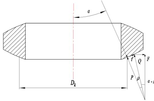
**Fig.4** Diagram of the force acting on the lenticular gasket
