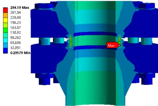
(d) Equivalent stress cloud diagram of the optimized sealing structure at 125°C
