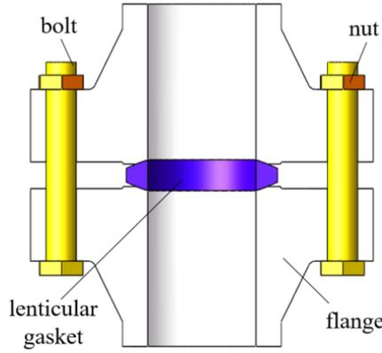
**Fig.1** Diagram of the offshore flange connector's structure
