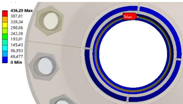
(a) Contact pressure cloud diagram of the non-optimized sealing structure at 25° C
