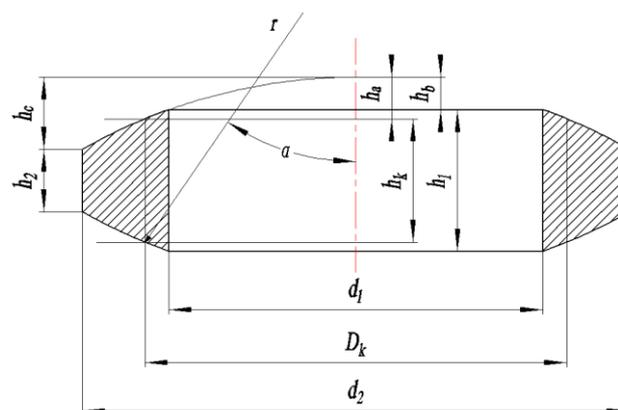
Fig.3 Structural design diagram of the lenticular gasket
