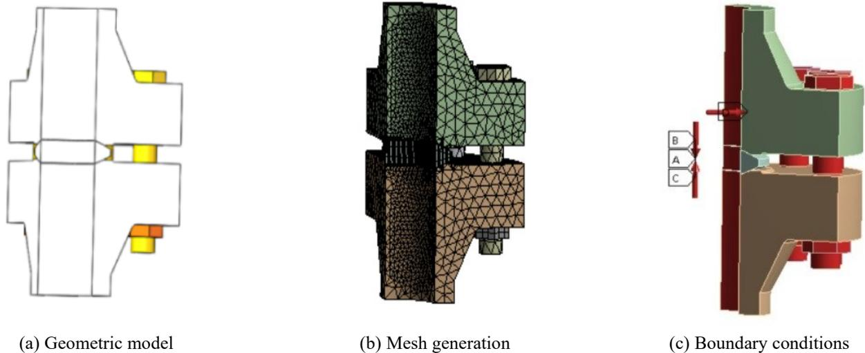
**Fig.7** Modeling of finite element analysis
