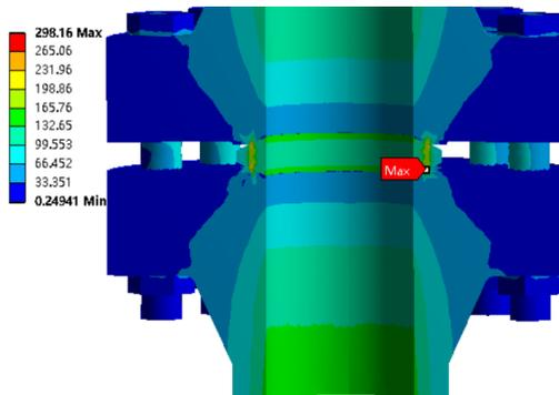
(d) Equivalent stress cloud diagram of the optimized sealing structure at 125°C
