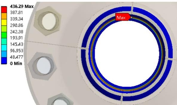
(a) Contact pressure cloud diagram of the non-optimized sealing structure at 25°C
