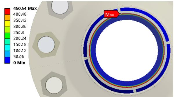
(b) Contact pressure cloud diagram of the optimized sealing structure at 25°C
