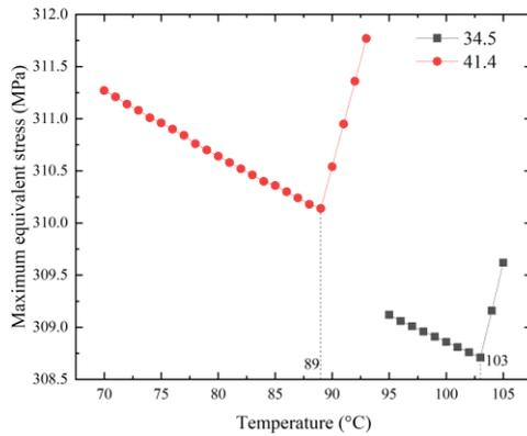
**Fig.16** The inflection point of the maximum equivalent stress of the non-optimized sealing structure
