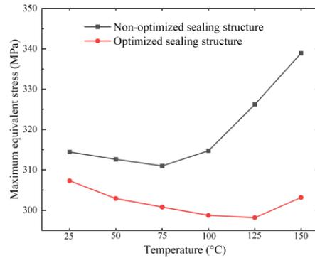
**Fig.15** Maximum Equivalent Stress diagram of non-optimized and optimized sealing structure under design pressure of 41.4 MPa
