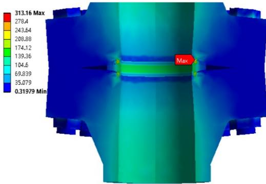
(a) Equivalent stress cloud diagram of the non-optimized sealing structure at 25°C
