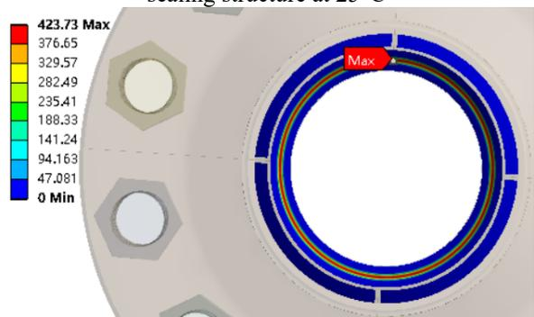
(c) Contact pressure cloud diagram of the non-optimized sealing structure at 125°C
