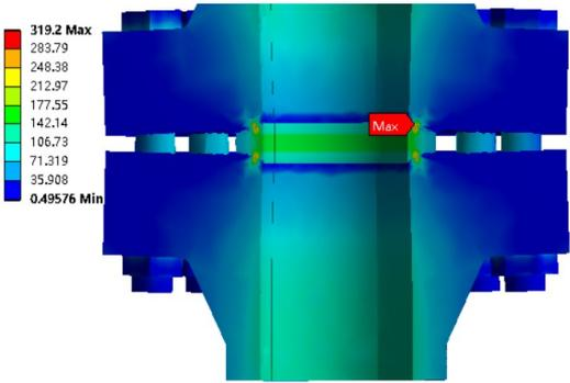
(c) Equivalent stress cloud diagram of the non-optimized sealing structure at 125°C
