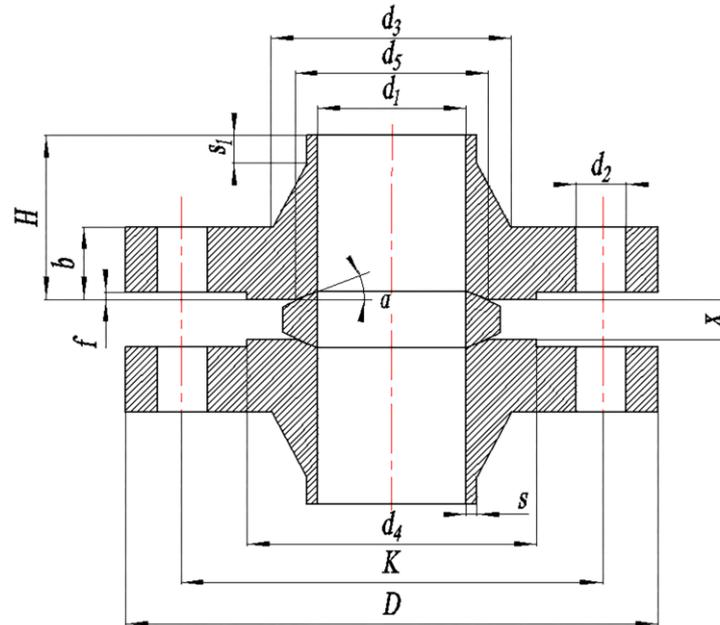
Fig.2 Structure design and assembly diagram of flange
