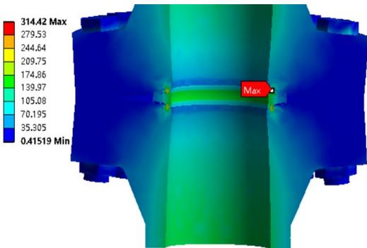
(a) Equivalent stress cloud diagram of the non-optimized sealing structure at 25°C
