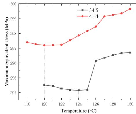
**Fig.17** The inflection point of the maximum equivalent stress of the optimized sealing structure
