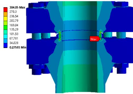
(b) Equivalent stress cloud diagram of the optimized sealing structure at 25°C
