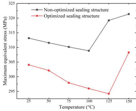
**Fig.14** Maximum Equivalent Stress diagram of non-optimized and optimized sealing structure under design pressure of 34.5 MPa
