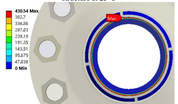
(d) Contact pressure cloud diagram of the optimized sealing structure at 125°C
