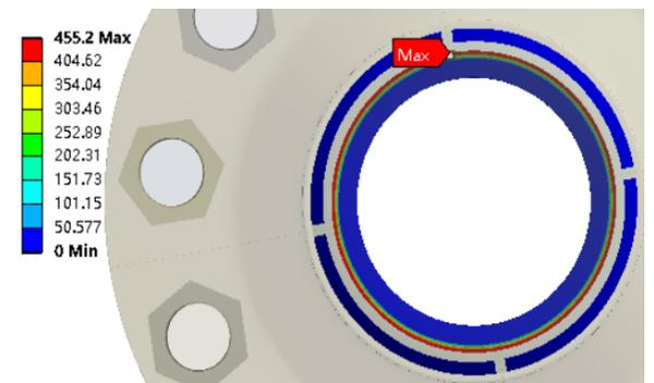
(b) Contact pressure cloud diagram of the optimized sealing structure at 25°C
