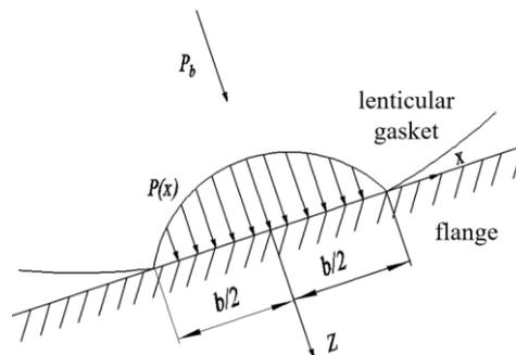
**Fig.5** Two-dimensional contact force between the flange and the lenticular gasket
