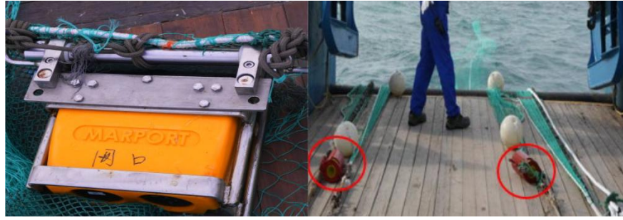
Fig. 8 Flow velocity and wing-end spread monitor
