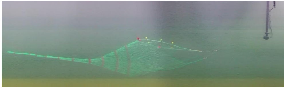
Fig. 5 Side view morphology of the net in the towing tank
