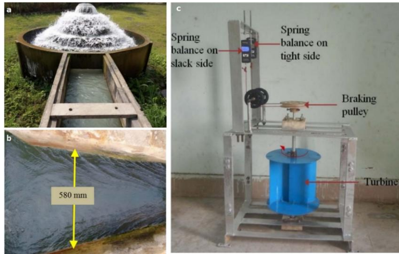
Fig. 3 Experimental flume setup: (a) the open channel with dimensions of 1 m width and 0.9 m height, and (b) the converging section (0.58 m width) where flow velocity was maintained at 0.8 m/s; (c) Overview of the experimental setup used to evaluate SHT performance [41]
