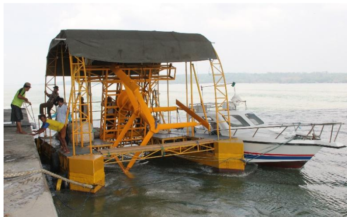
Fig. 16 BRIN vertical-axis ocean current turbine prototype conducted in 2014 [43]
