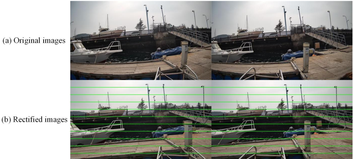
Fig. 10 Stereo image rectification results
