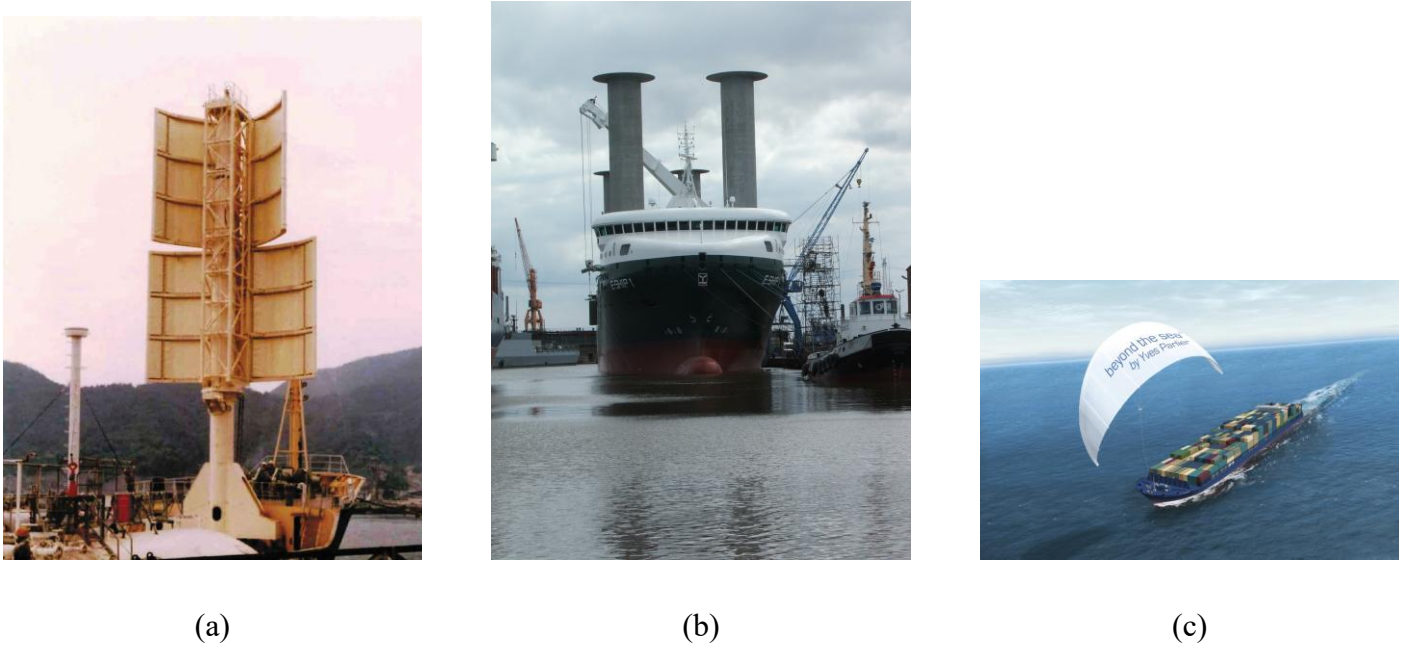
Fig. 3 Real-world applications of Wind-Assisted Ship Propulsion (WASP) technologies: (a) Shin Aitoku Maru equipped with rigid wing sails [36] (CC BY 4.0); (b) E-Ship 1 with rotor sails (CC BY-SA 3.0); (c) container ship towed by a kite sail from Beyond the Sea[37] (CC BY-SA 4.0)
