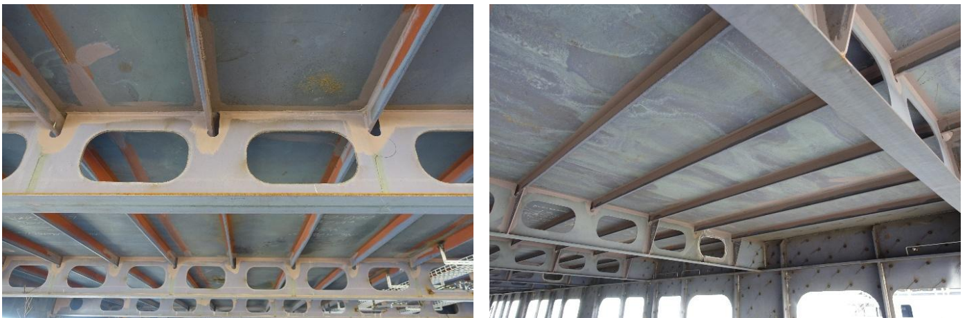
Fig. 2 Typical ship deck stiffened structure
